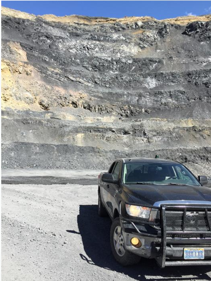
Open pit benches with exposed mineralization
