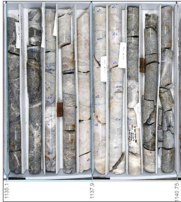
Figure 3: Core Photography of the Navidad Vein with High-Grade Gold and Silver Mineralization detected by XRF Analyzer. Hole EW-24-372A Assay Results: 3.24 m at 13.06 g/t Au and 206 g/t Ag.
