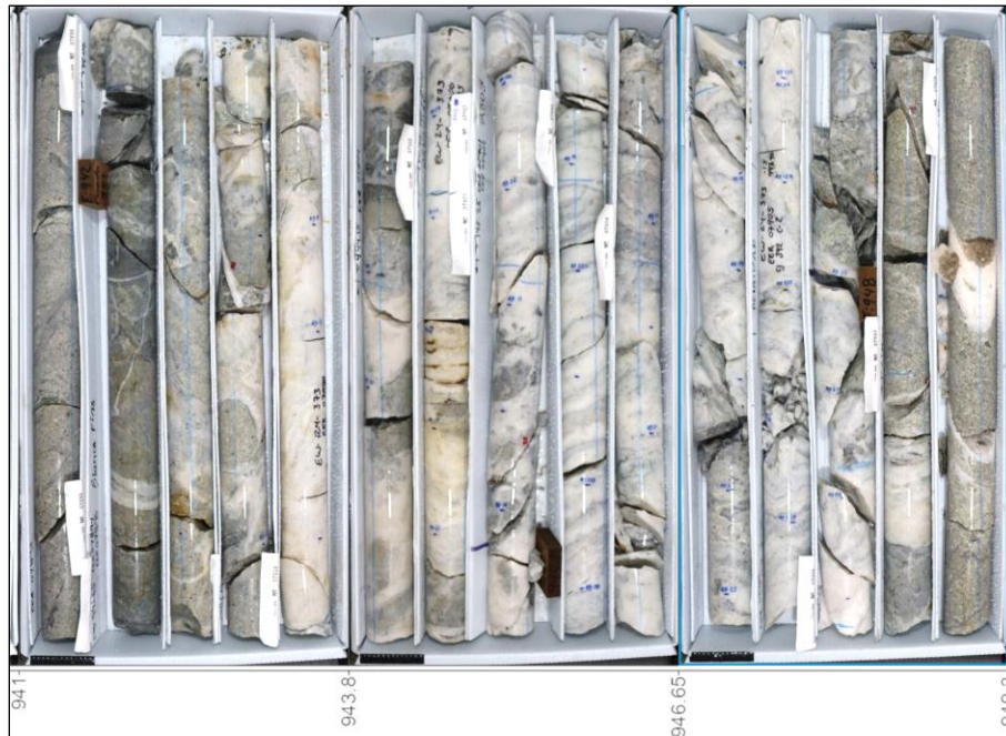
Figure 2: Core Photography of the Winter Vein with High-Grade Gold and Silver Mineralization detected by XRF Analyzer. Hole EW-24-373 Assay Results: 6.06 m at 5.64 g/t Au and 104 g/t Ag.
