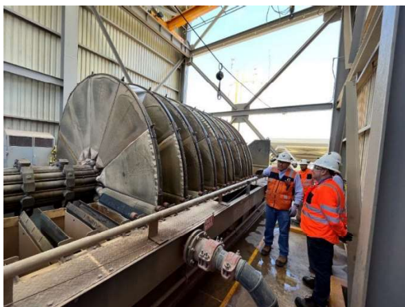
Figure 18.10: Tailings Dewatering Disc Filter (left) and Positive Displacement Pumps for Paste Fill (right)
