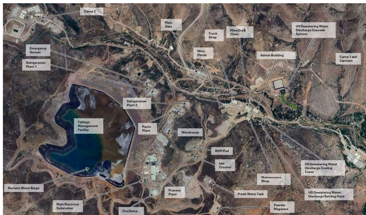
Figure 18.2: Aerial View of Overall Site with Infrastructure in As-Built Conditions
