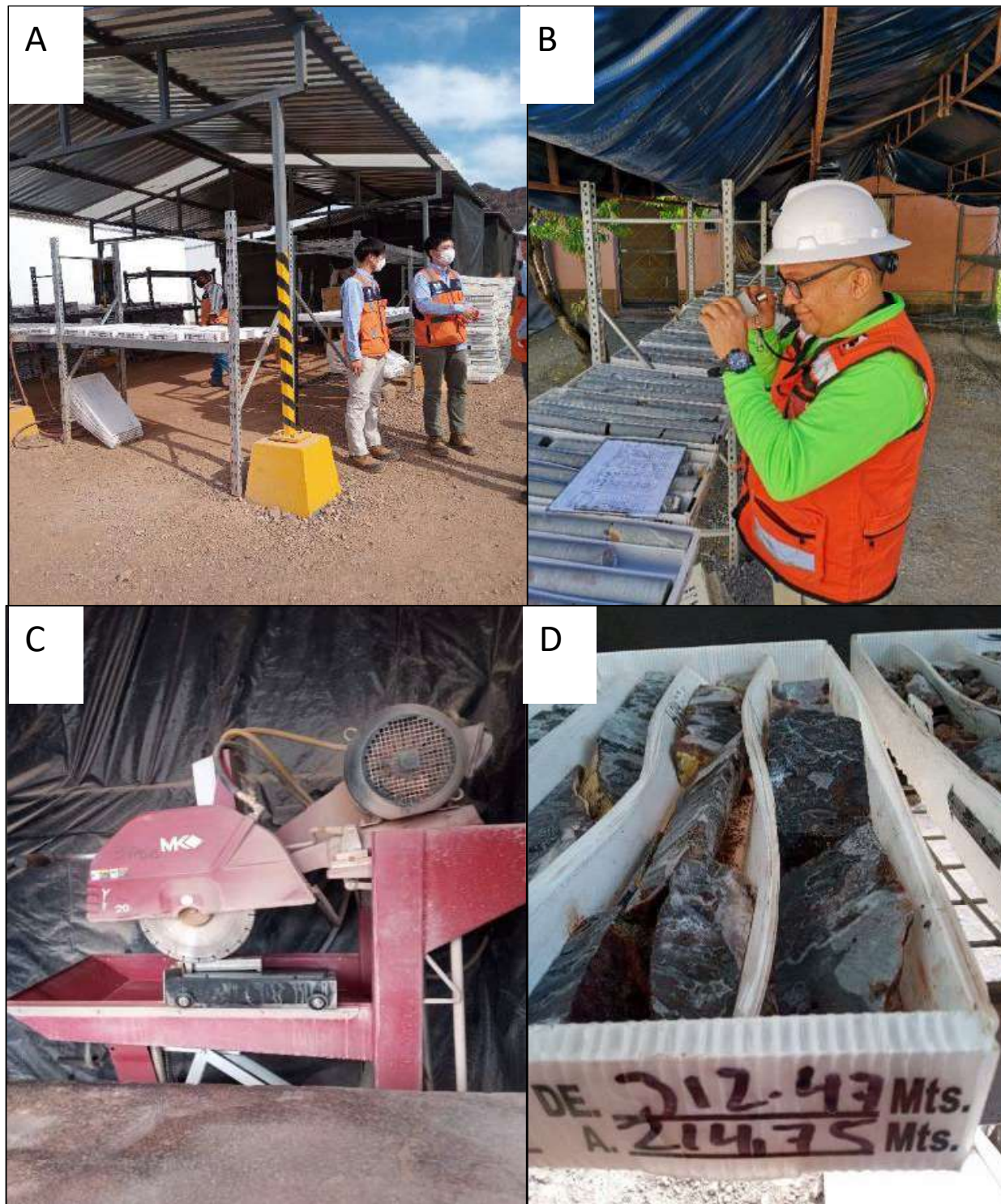
Figure 11.2: A) Geological Core-Shack; B), Geological Logging on Site; C), Electrical Diamond Saw; D), Half Core Placed in a Labelled Core Box
