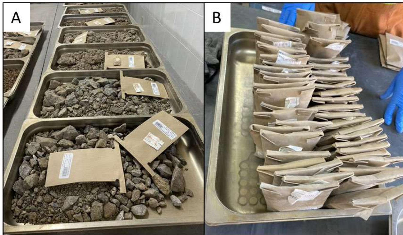
Figure 11.5: Samples After Crushing (Left) and Pulp Samples Labelled (Right)
